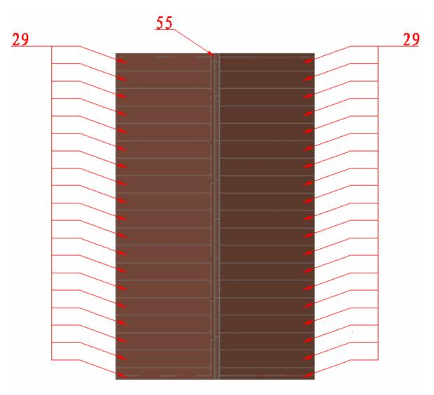
Note: when install the front and back panels, please install the color steel plate from the middle to the sides
